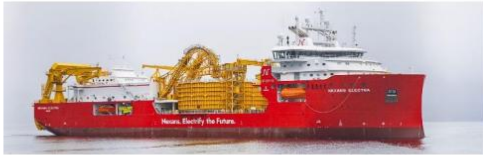
Nexans Electra – constructs 4 drum vessel
