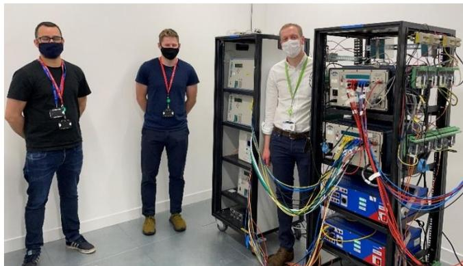
By bringing together the Replica of the CMS control scheme with actual protection relays (pictured above) with our extensive real-time model of the island's network, we can thoroughly test the robustness of the overall system during fault conditions.
