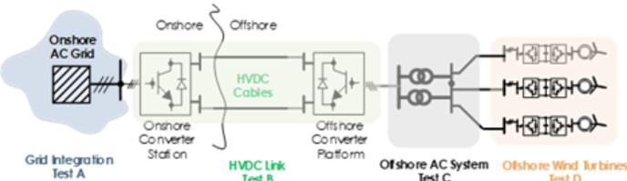
Fig: HVDC-connected offshore wind farm
