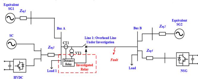
We recently hosted a joint webinar with Strathclyde where we reported on the project that we ran looking at evaluation of HVDC impact on AC network protection. This project provides a great RTDS HIL platform to test the operation of protection relays for a easily customisable mix of HVDC convertor, traditional fault levels and renewable energy sources.
