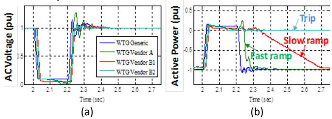
Fig: Simulation results for a 3-phase to ground offshore AC fault F1 for 4 different wind farm models. (a) offshore AC voltage (pu); (b) active power (pu). Adapted from the [full report](#) [2].
