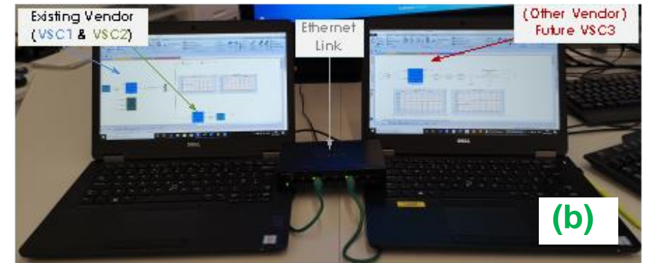
Fig. 2: Co-simulation of 3-terminal HVDC Scheme (a) Schematic. (b) Set-up.
