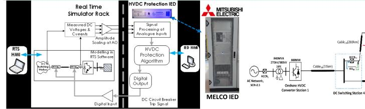
Converter Station Real time Simulation Test Setup & Schematic Diagram
