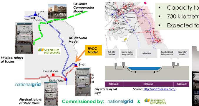
Overview of Eccles-Blyth-Stella West 400kV Protection Performance Studies Capacity to transmit 1,400 MW of power at DC voltage ±525kV
