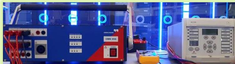
This was achieved by amplifying the current and voltage signals from RTDS® I/O cards using an amplifier which was further injected to the AC Protection relay. Such a setup will be used in the innovation project which the Centre is sponsoring with EPRI. The power amplifier setup (with RTDS®) will also be used to support future testing of protection relays in collaboration with transmission operators for the upcoming HVDC projects in the GB Network.
